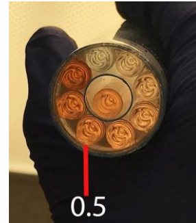
Picture 1: CHEMetrics® Color Comparator at 0.5 ppm
